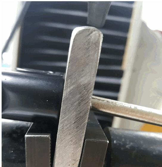
Type of failure observed: Pin deformed. Pin was able to be removed from lock
